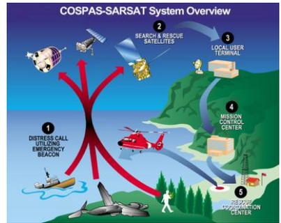
The LUT processes the Doppler-shifted signal from the LEOSAR and determines the location of the beacon, then the LUT relays the position of the distress to a Mission Control Center (MCC) where the distress alert and location information is immediately forwarded to an appropriate Rescue Coordination Center (RCC). The RCC dispatches Search and Rescue (SAR) forces.
