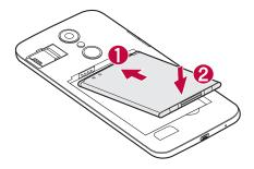
4 To replace the cover onto the device, align the back cover over the battery compartment and press it down until it clicks into place.
