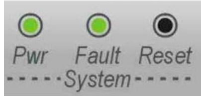
Figure 11: System - AN-100U/UX System LEDs and Reset Switch
