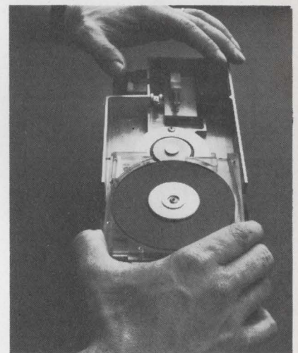
Figure 1: The SQ306 from Syquest Technology offers 5 Mbytes of storage in a 100mm removable cartridge drive.
