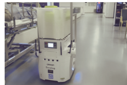
Mobile robots that transport medical waste at hospitals in Finland
