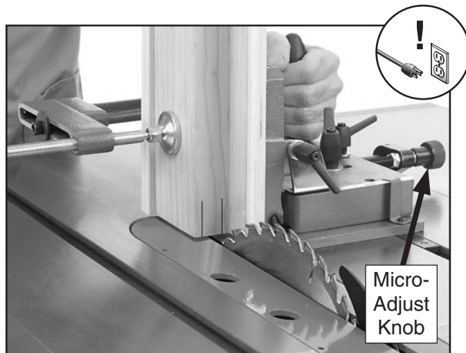
Figure 28. Aligning workpiece for first structural cheek cut.
