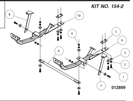
**IMPORTANT:** All baseplates **must** be assembled with all the bolts left loose for final adjustment and positioning (before tightening) unless otherwise instructed. All bolts **must** be torqued for proper strength. If more than one bolt is used per fastening point, the diagram may only show one.
