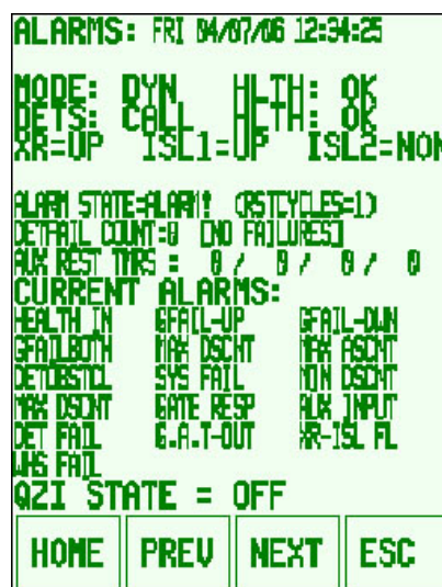
Figure 3-9 Typical Alarm Status Display
