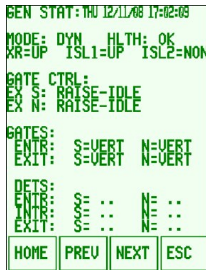
Figure 3-6 Typical General Status Display
