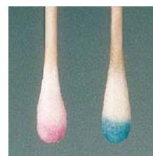
Nitrate swab with positive (left) and negative (right) reactions.
