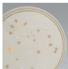
Tryptic Soy Agar Settling Plate w/growth.
