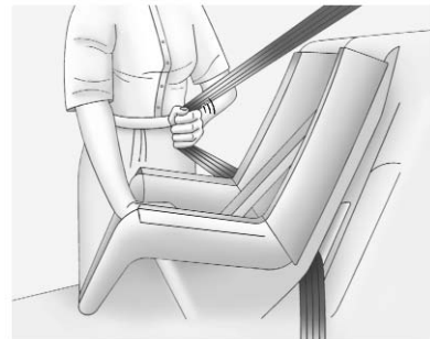
Tilt the latch plate to adjust the belt, if needed.
