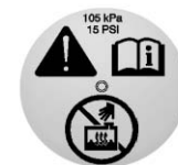
Light-Duty Coolant Surge Tank Pressure Cap
