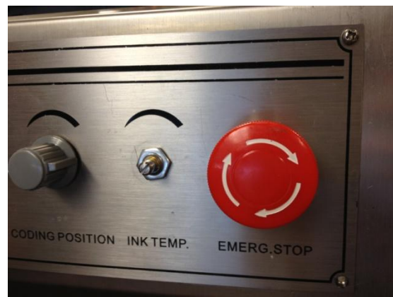
Figure 28. Remove Washer Holding Ink Temperature Potentiometer
