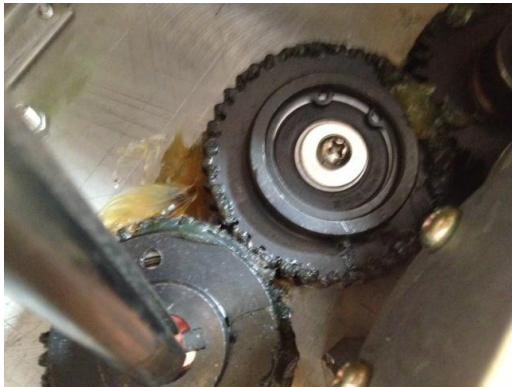
Figure 5. Ensure the groove in the long shaft matches that in the gear
