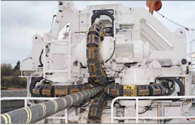
6 The cable tensioner (on board the laying vessel)
