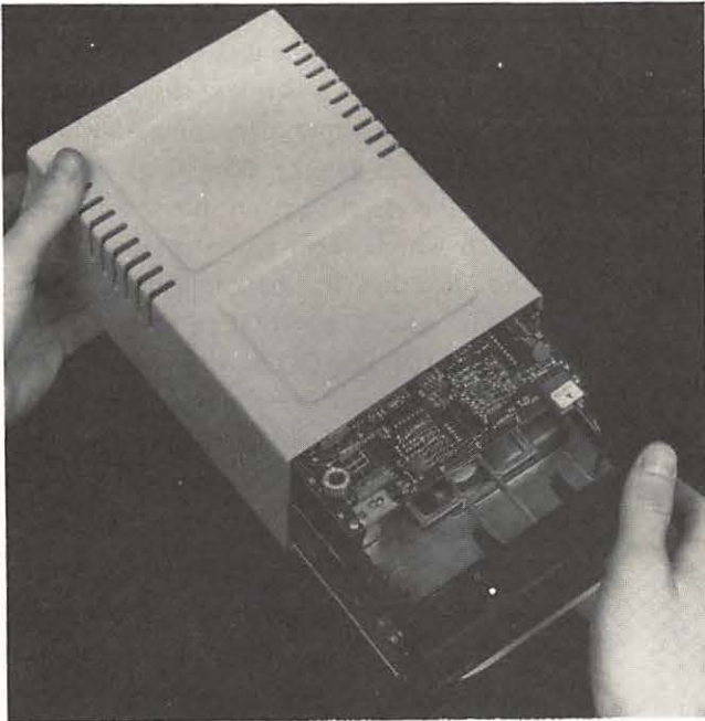
Fig. 8-19. Gently slide the drive cover housing back off the drive mechanism.
