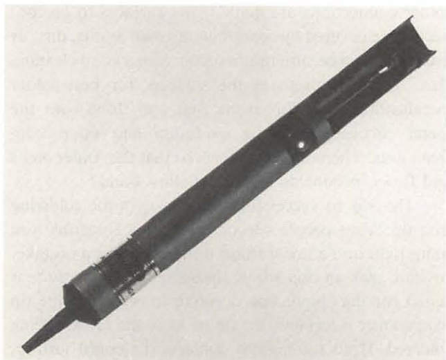
Fig. 9-22. The spring-driven plunger in the solder vacuum pump is used to pull hot solder off a connection.
