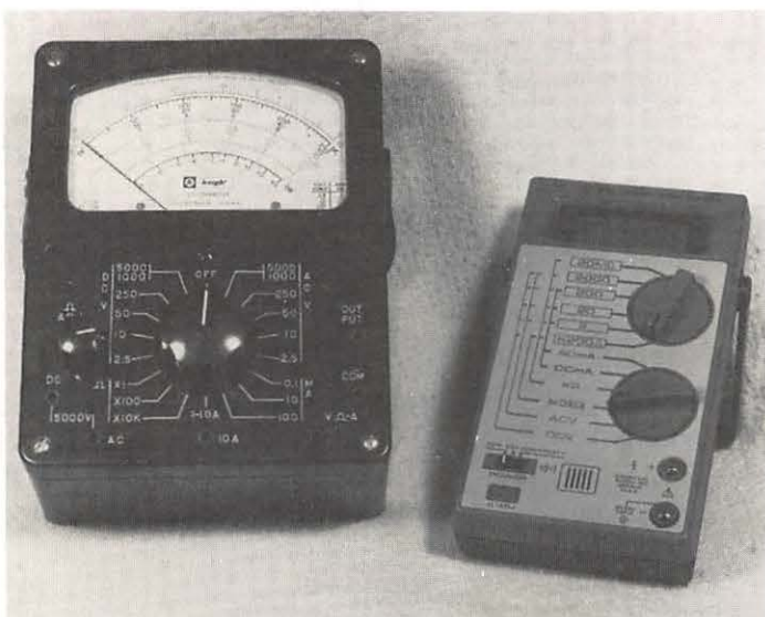
Fig. 9-1. A volt-ohm-milliammeter (VOM) and a digital voltmeter (DVM).
