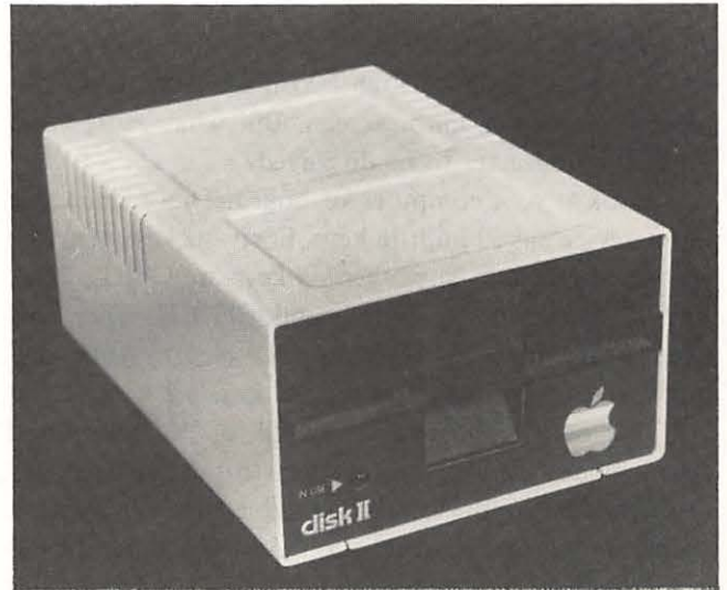
Fig. 3-19. The Disk II is the drive most commonly used with the Apple II Plus computer.
