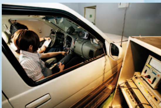
Shield Room for Vehicle
