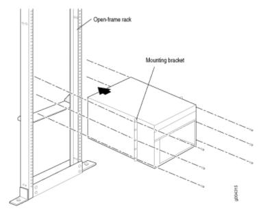
**NOTE**: This illustration depicts the router being installed in an open-frame rack. For an illustration of the mounting hardware required for a four-post open rack or open cabinet, see "Installing the MX240 Router Mounting Hardware for a Rack or Cabinet" on page 227.
