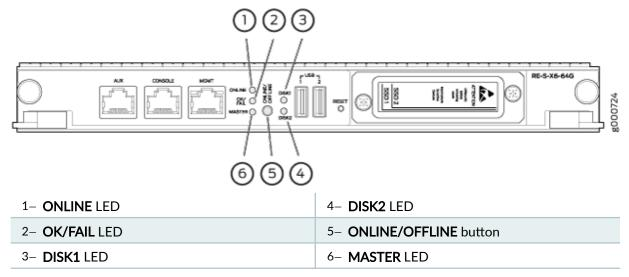
Table 26: RE-S-X6-64G Routing Engine LEDs
