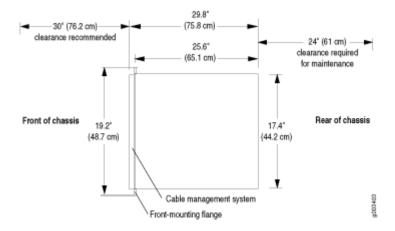
Figure 47: Chassis Dimensions and Clearance Requirements
