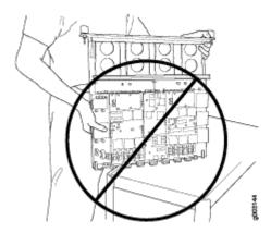
You hold an FPC horizontally when installing it into the chassis or an equipment rack. To hold an FPC vertically (see Figure 115 on page 345):
