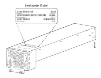
Figure 158: DC Power Supply Serial Number Label
