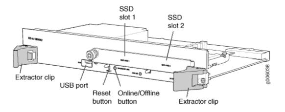
Figure 27: RE-S-X6-64G Routing Engine Front View
