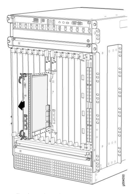
Figure 99: Removing a Routing Engine from an MX960 Router
