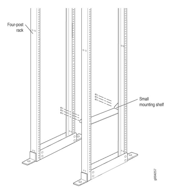
Figure 51: Installing the Mounting Hardware for an Open-Frame Rack
