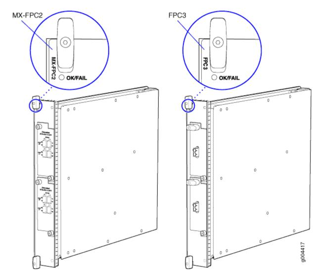
Figure 37: Typical FPCs Supported on the MX240 Router
