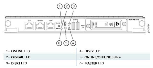
Table 23: RE-S-X6-128G Routing Engine LEDs
