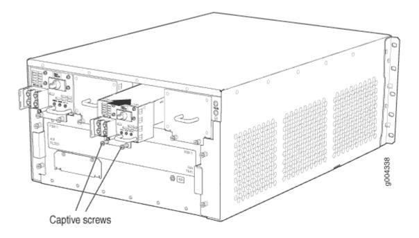
Figure 140: Connecting DC Power to the Router
