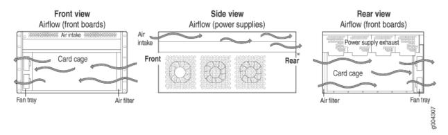
The host subsystem monitors the temperature of the router components. When the router is operating normally, the fans function at lower than full speed. If a fan fails or the ambient temperature rises above a threshold, the speed of the remaining fans is automatically adjusted to keep the temperature within the acceptable range. If the ambient maximum temperature specification is exceeded and the system
