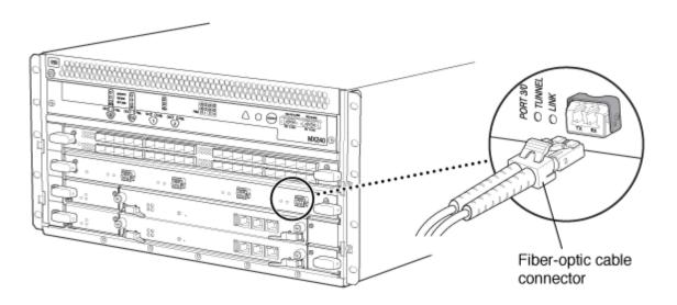
Figure 83: Attaching a Cable to a MIC
