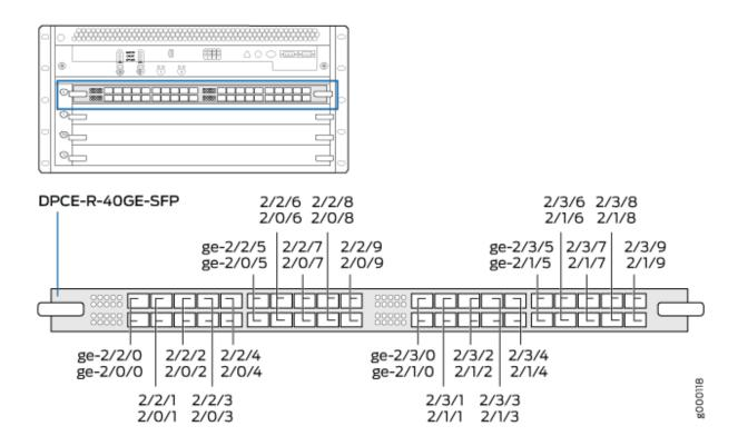
The DPC contains four logical PICs, numbered PIC 0 through PIC 3 in the CLI. Each logical PIC contains 10 ports numbered 0 through 9.
