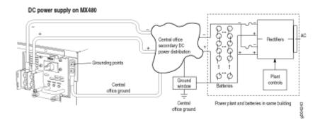
The DC power supply in **PEM0** must be powered by a dedicated power feed derived from feed **A**, and the DC power supply in **PEM2** must be powered by a dedicated power feed derived from feed **B**. This configuration provides the commonly deployed **A/B** feed redundancy for the system.
