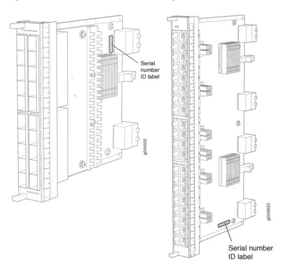
Figure 153: 20-Port MIC Serial Number Label
