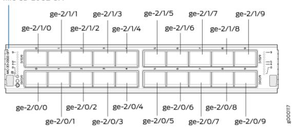
The MIC contains two logical PICs, numbered PIC 0 through PIC 1 in the CLI. Each logical PIC contains 10 ports numbered 0 through 9.
