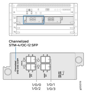
The show chassis hardware command output displays a Channelized OC12/STM4 Enhanced IQ (IQE) PIC (4x CHOC12 IQE SONET) installed in MX FPC Type 2.
