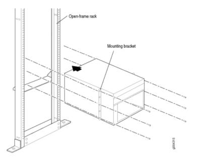
**NOTE**: This illustration depicts the router being installed in an open-frame rack. For an illustration of the mounting hardware required for a four-post rack or cabinet, see "Installing the MX240 Router Mounting Hardware for a Rack or Cabinet" on page 227.
