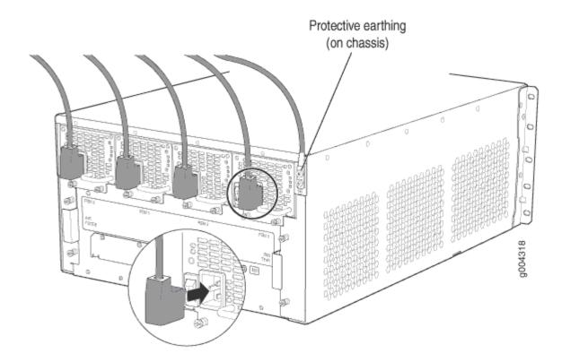
Figure 20: Connecting DC Power to the Router
