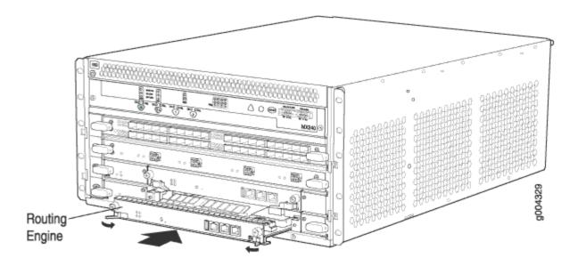
Figure 101: Installing a Routing Engine in an MX480 Router
