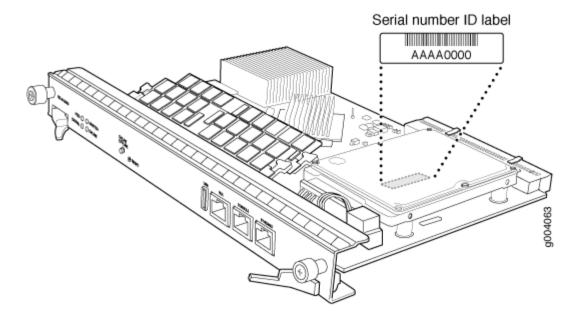
Figure 160: RE-S-X6-64G Routing Engine Serial Number Label
