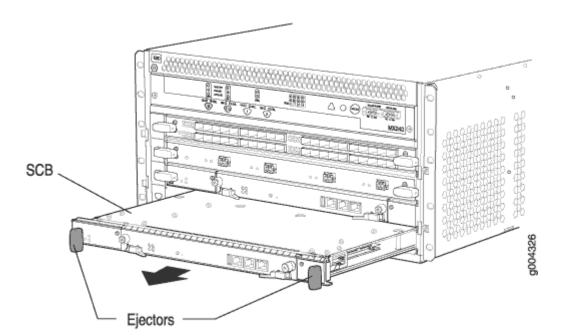
Figure 143: Removing the Switch Control Board from an MX240 Router
