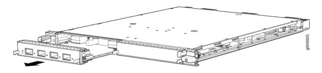
Figure 120: Removing a Dual-Wide MIC
