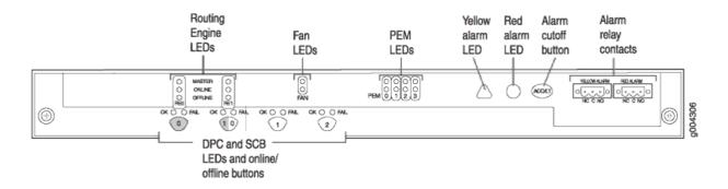
NOTE: At least one SCB must be installed in the router for the craft interface to obtain power.
