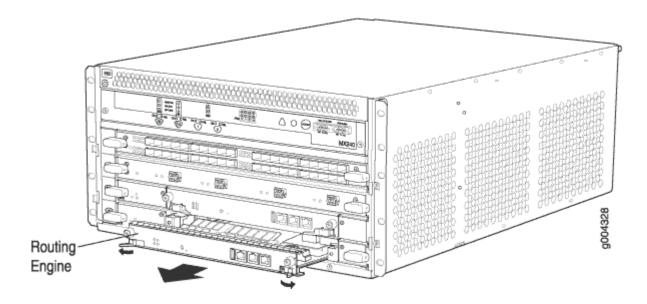
Figure 98: Removing a Routing Engine from an MX480 Router
