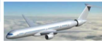
Bauhaus Luftfahrt "Propulsive Fuselage" Thrust split 77/23
