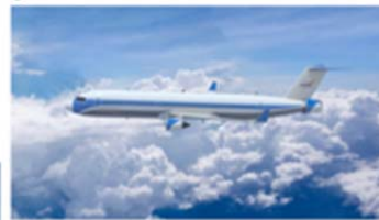
NASA STARC-ABL Thrust split: 84/16 takeoff 56/44 cruise
