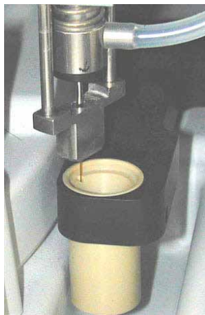
Fig. 49: Fused silica needle in wash port
