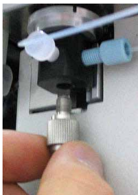
Fig. 44: Removing the syringe from the syringe valve
