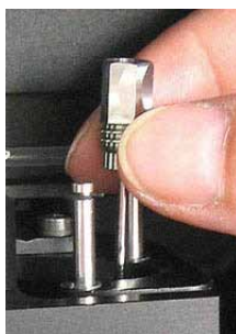
Fig. 53: Removing the puncturer
