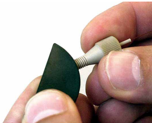
Fig. 66: Preassembling the fitting connection
