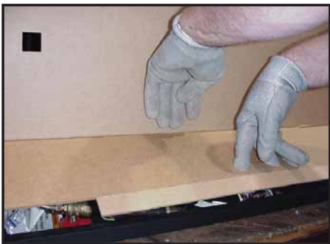
Figure 13.8 Opening Lower Access Panel
