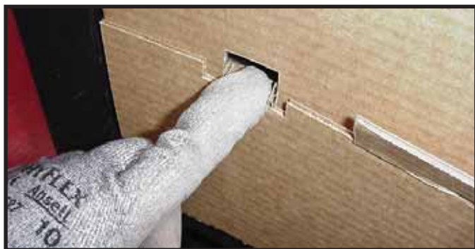
Figure 13.9 Securing Tabs Inside Front of Splatter Guard
