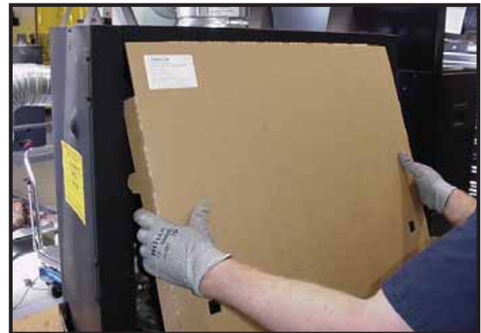
Figure 13.4 Installation of Splatter Guard
