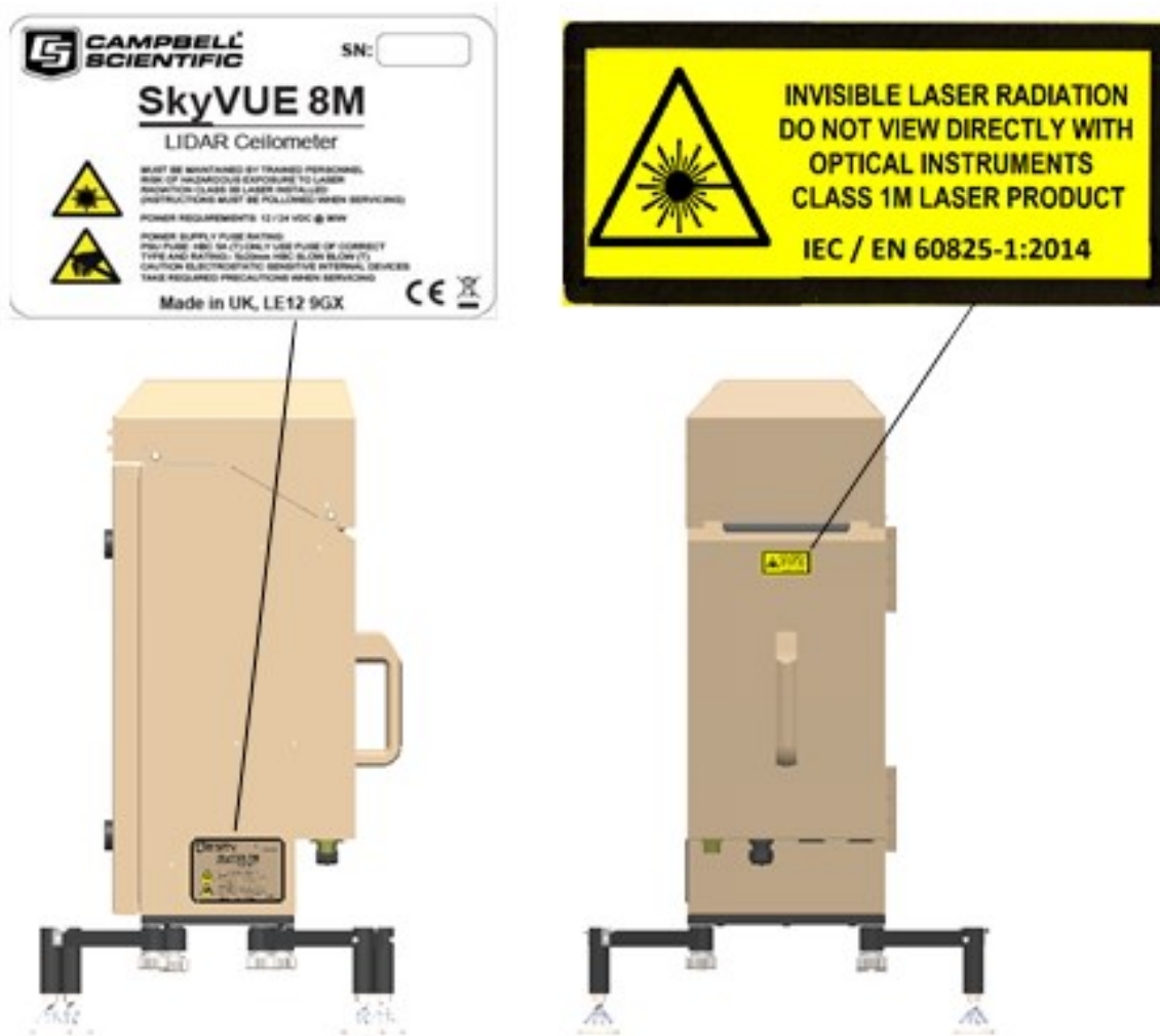
FIGURE 1-1. Location of laser warning label
