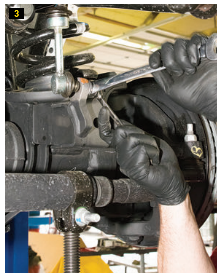
1) Ram went to the three-link coil front suspension in the 2014 2500 4x4s. The following year Ram 3500s received the same suspension upgrade. Epiq's leveling kit fits 2014 Ram 2500 4x4s and 2015 and newer 2500/3500 4x4s. 2) The first step is to remove the lower bolts from the front shocks with jack stands supporting the front axle. 3) The front sway bar is disconnected from the drop links using a 10mm wrench to hold the pin and a 21mm socket to remove the nut. Disconnecting the track bar isn't necessary, but doing so will make the upgrade easier if you are working without the benefit of a hoist.
