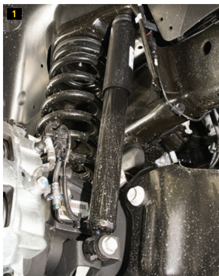
1) Ram went to the three-link coil front suspension in the 2014 2500 4x4s. The following year Ram 3500s received the same suspension upgrade. Epiq's leveling kit fits 2014 Ram 2500 4x4s and 2015 and newer 2500/3500 4x4s. 2) The first step is to remove the lower bolts from the front shocks with jack stands supporting the front axle. 3) The front sway bar is disconnected from the drop links using a 10mm wrench to hold the pin and a 21mm socket to remove the nut. Disconnecting the track bar isn't necessary, but doing so will make the upgrade easier if you are working without the benefit of a hoist.
