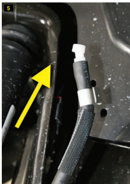
4) Before the axle housing is lowered, the brake-line bracket on each side is disconnected at the base of the coils, so the hoses don't get stretched or damaged. 5) The differential breather tube is disconnected from its retainer clip on the upper rear of the driver's-side coil tower. 6) After the brake line and breather hose are free, the axle housing is slowly lowered until the top of the front coil on each side can be easily pulled out from the upper bracket. 7) The Epiq spacer (same for both sides) is placed on top of the coil's rubber isolator and rotated so it aligns with the top bucket mount. The spacer is offset toward the rear of the truck.
