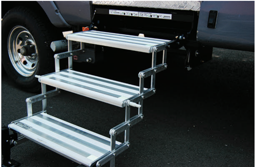
The near-effortless scissor-type mechanism allows the steps to be adjusted to accommodate various heights from the ground. A three-step model was installed on the test trailer; systems are also available with two, four, five or six steps.
