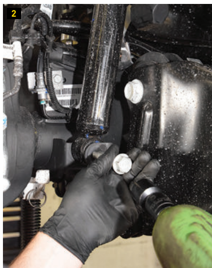
1) Ram went to the three-link coil front suspension in the 2014 2500 4x4s. The following year Ram 3500s received the same suspension upgrade. Epiq's leveling kit fits 2014 Ram 2500 4x4s and 2015 and newer 2500/3500 4x4s. 2) The first step is to remove the lower bolts from the front shocks with jack stands supporting the front axle. 3) The front sway bar is disconnected from the drop links using a 10mm wrench to hold the pin and a 21mm socket to remove the nut. Disconnecting the track bar isn't necessary, but doing so will make the upgrade easier if you are working without the benefit of a hoist.
