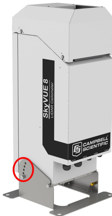
FIGURE 4-2. Setting the tilt angle
