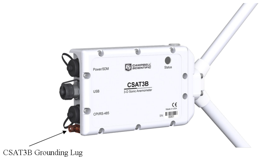
FIGURE 4-3. Grounding lug of CSAT3B
