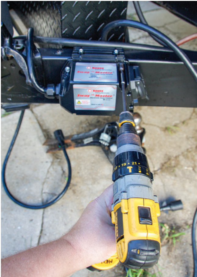
(Above left) Installing the Sway Master is simple. Four self-drilling screws secure it to the frame. (Above right) The trailer's seven-way cable plugs into the unit. The cable is routed to the front and secured using cable clips, and the LP-gas line is resecured.
