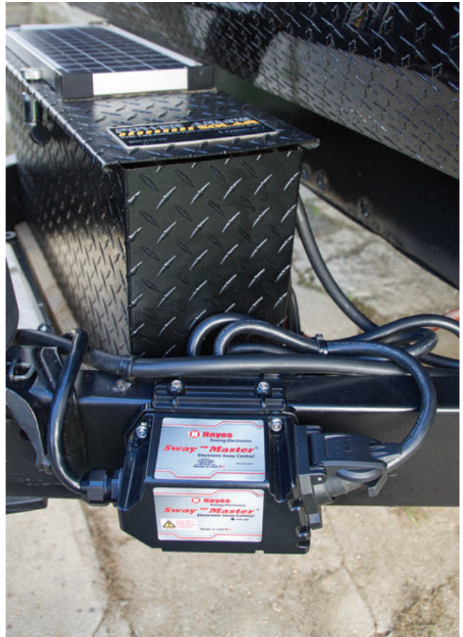
(Above left) Installing the Sway Master is simple. Four self-drilling screws secure it to the frame. (Above right) The trailer's seven-way cable plugs into the unit. The cable is routed to the front and secured using cable clips, and the LP-gas line is resecured.
