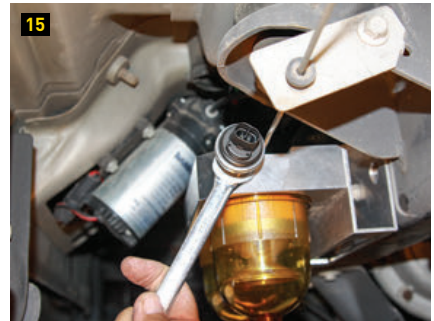
(14 and 15) The optional Filter Minder warning-light electronic sending unit is installed in the base assembly after removing the plug with an Allen wrench.
