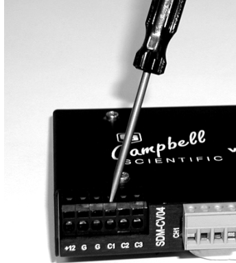
FIGURE 7-1. Use of the Spring-Loaded Terminal Blocks (Top Position)
