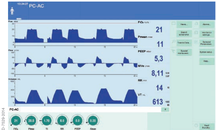
Fig. 2 (PC-AC with triggered and untriggered mechanical breaths)
