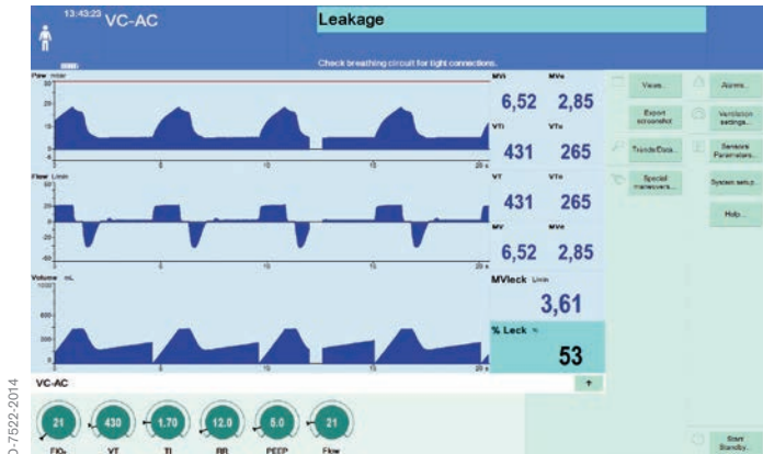
Fig. 1 Screen example with VC-AC, large leak without leak compensation
