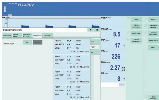
Fig. 2 Screen example of the intrinsic PEEP measurement
