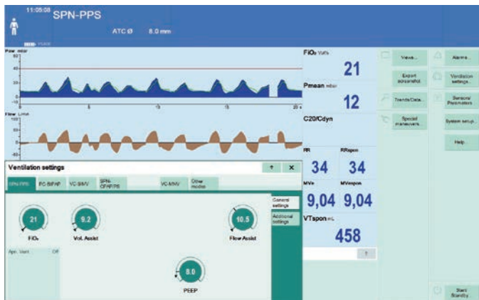
Fig. 2 SPN-PPS, typical pressure and flow graph
