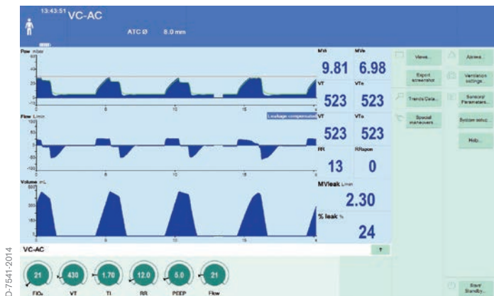
Fig. 2 Screen example with VC-AC, large leak with leak compensation
