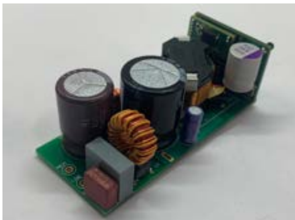
Figure 2. A 65-W active clamp flyback converter measuring 65 mm by 28 mm by 25 mm.
