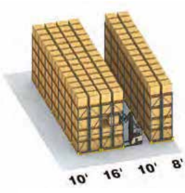
Double-Deep Rack Double Reach Lift Truck 8.5'-11' aisle width
