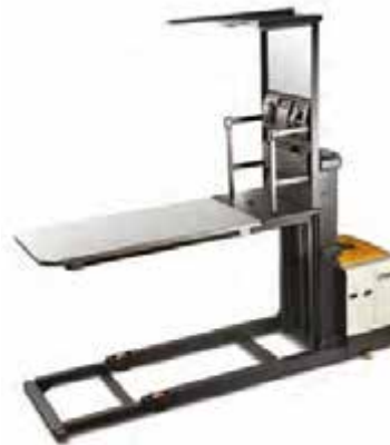
SP 3570F Series Straddle Load Capacity: 3000 lbs. Lift Height: 210 to 366 in.
