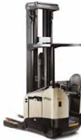
RR 5700S Series Load Capacity: 4500 lbs. Lift Height: 198 to 442 in
