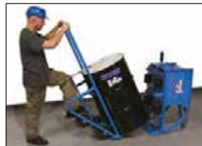
Place your drum onto the base plate of the 55-gallon drum mixer with a drum truck or a hook drum lifter.
