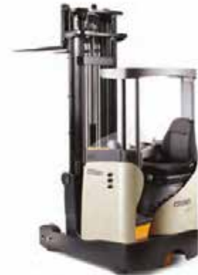
ESR 5200 Series Load Capacity: 3000, 3500 & 4500 lbs. Lift Height: 108 to 511 in.
