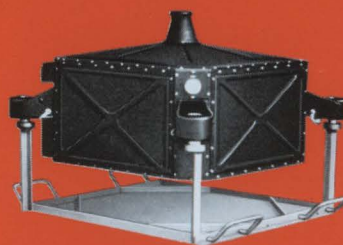
Saturn I guidance computer continuously determined the v course to achieve orbit. In six test flights, these computer NASA Saturn I vehicle controlled the direction and thrus second-stage engines. The computer on four of the flights co four of the first-stage engines as well, and also timed engine
