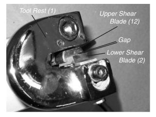
4. Loosen the Socket Head Screw (6) that holds the Upper Shear Blade (12) in place. Adjust the Upper Shear Blade until the space between the upper and lower cutting edge is between 0.1 mm and 0.6 mm. Then tighten the Socket Head Screw (6) to fix the Upper Shear Blade (12) in position.
