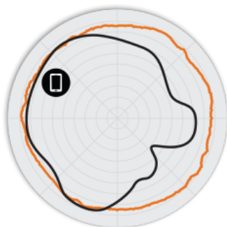
Figure 2. R320 2.4GHz Azimuth Antenna Patterns
