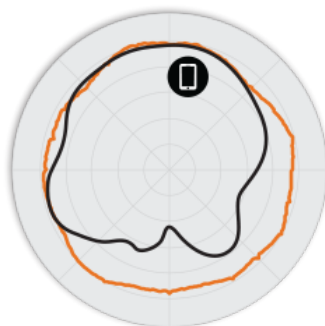
Figure 3. R320 5GHz Azimuth Antenna Patterns
