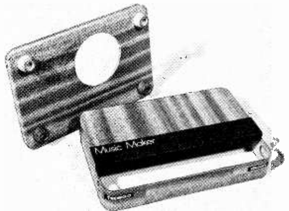
The case used for the prototype—the black escutcheon can be made from cardboard covered with black, self-adhesive plastic.
