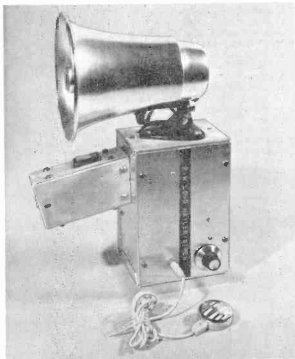
The loudhailer need not be hand held and can be rested as shown with the speaker adjusted to face forwards.
