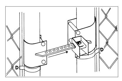
Note: When gates are in a closed position, latch can now be padlocked through aligned holes.
