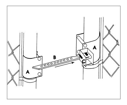
NOTE: Rotating enables latch pieces to slide into one another at the correct alignment.
