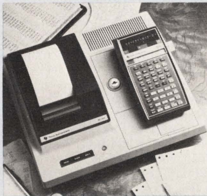
Texas Instruments SR-52 programmable calculator is converted into a desktop printing unit.
