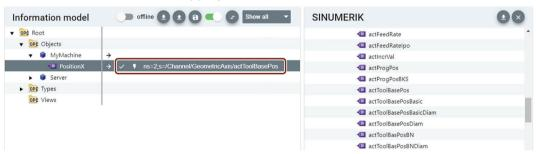
Figure 4-17 SINUMERIK variable added in mapping table
