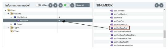
Figure 4-16 Mapping SINUMERIK variable
