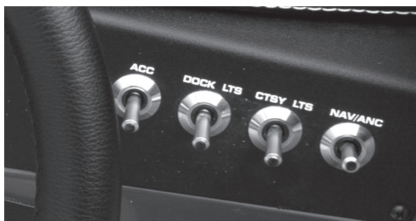
Figure H7: Helm Switch Panel - Starboard View (Representative View - Models May Vary)
