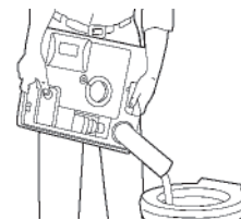
Figure J15: Emptying Waste Holding Tank
