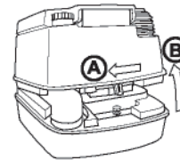
Figure J14 Removing Fresh Water Tank
