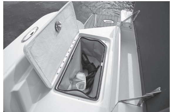
Figure L14: Transom Walk-thru Storage (Note: Meshed-sided Bag for Wet Gear)
