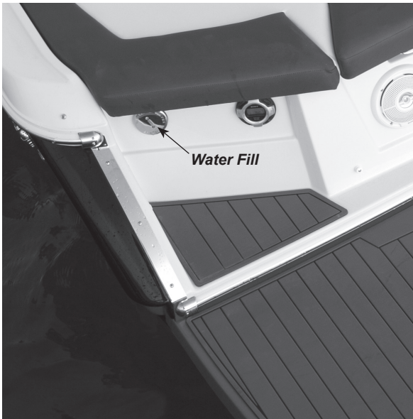
Figure J2: Water Fill - Port Transom
