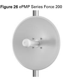
The Force 200 integrated dish is a selfcontained transceiver unit that houses both radio, parabolic dish and networking electronics. An ePMP Force 200 unit may function as an Access Point (AP) or a Subscriber Module (SM) in a Point-To-Multipoint (PMP) or in a Point-To-Point (PTP) network topology. It is typically deployed as an SM in a PMP system and either Master or Slave in a PTP system.
