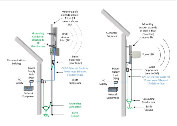
Figure 4 AP Cabling Diagram
