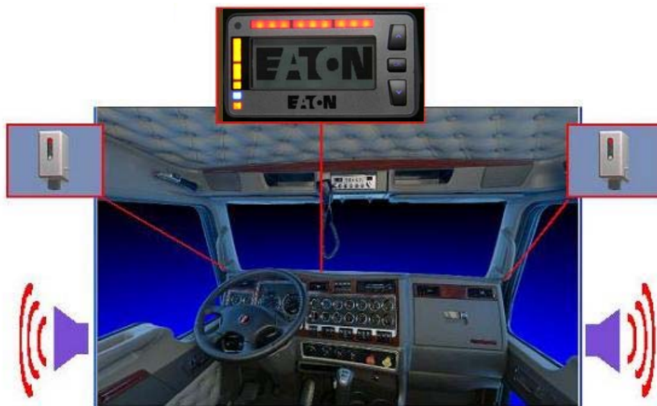
Figure 35. Heavy-truck DVI space in truck cockpit
