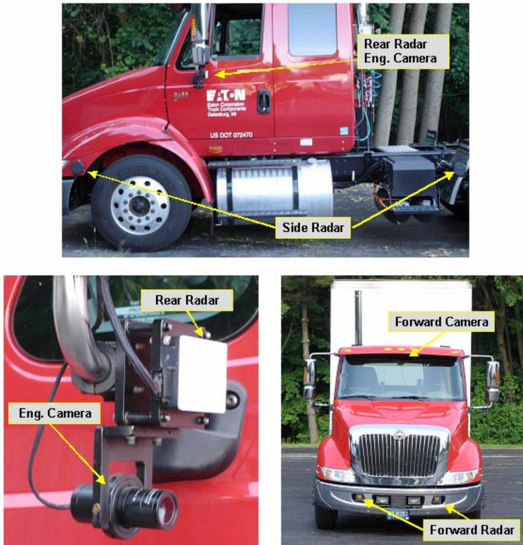
Figure 32. Bronze tractor sensor mounting
