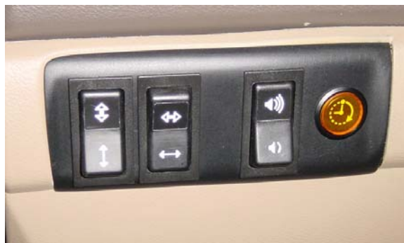
Figure 18. IVBSS mute button (right) and volume control switch (second from right)
