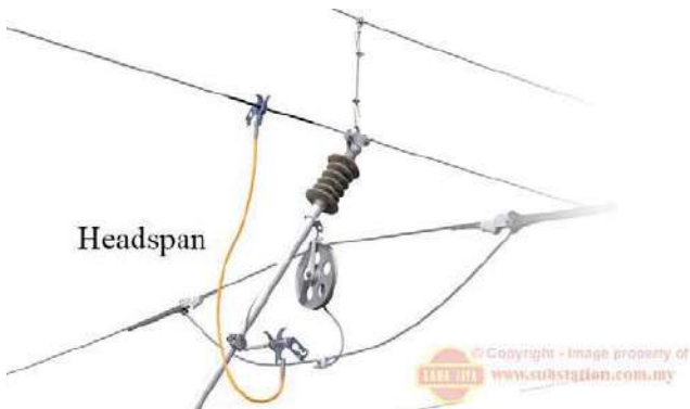
Headspan using Single Short Rail Earth
