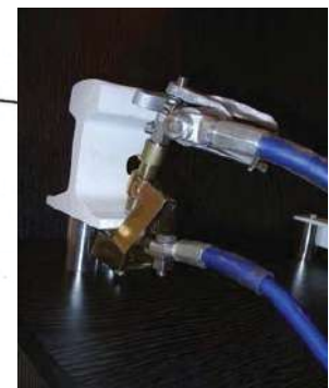
Interlocked clamps being applied to Flat bottom Rail Section
