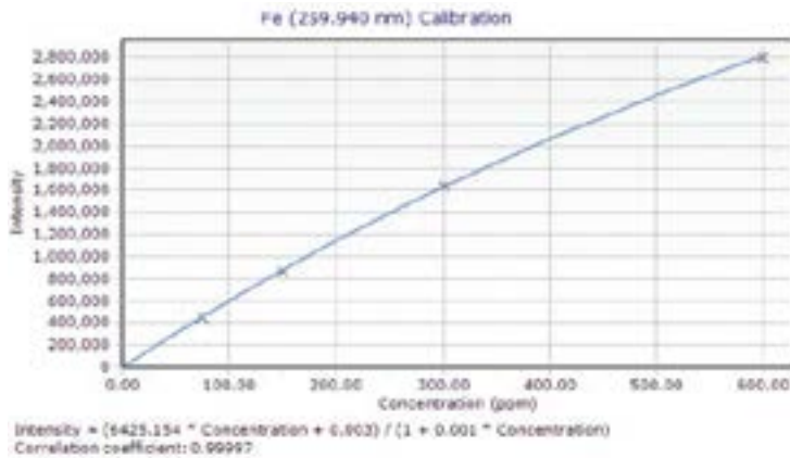
Figure 2. A typical non-linear calibration curve in MP-AES
