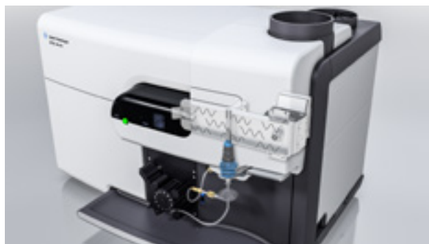
Figure 2. A microwave waveguide creates concentrated electromagnetic fields around the torch.
