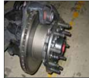
Steer Axle: Vented Air Disc Brake
