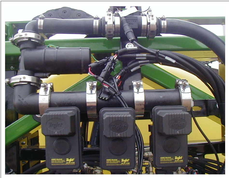
Fig. 4 CHEMICAL CIRCUIT CONTROLS
