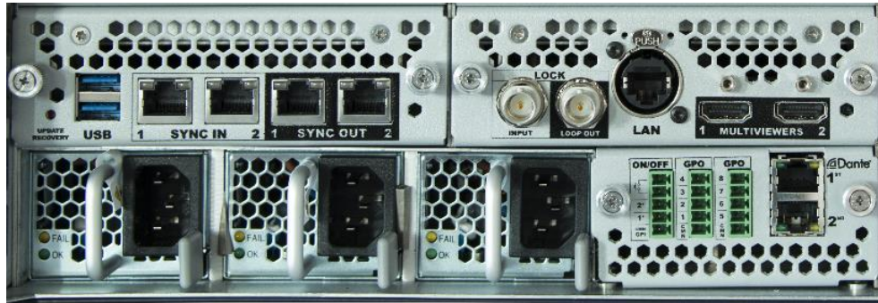
Fig. 3 - Fixed parts on all LivePremier units
