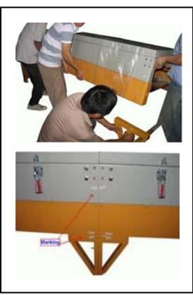
b) Move the heating chamber onto the 2 pedestals matching corresponding marks on pedestal and chamber.
