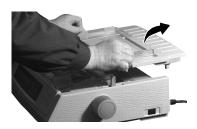
4 Fold some continuous-form paper over three times to make a page four sheets thick. Then, load it on the tractors and close the covers.
