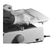
Pull up on the lock levers and open the tractor covers.
