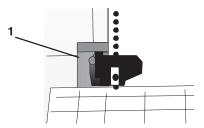
Adjust the position of the right tractor to center the holes in the paper on the pins. Then, push back the right lock lever.
