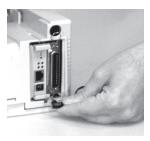
Attach the 10/100 Base-T UTP cable to the receptacle on the back of the OkiLAN 6120e. Attach the other end of the cable to the Network.
