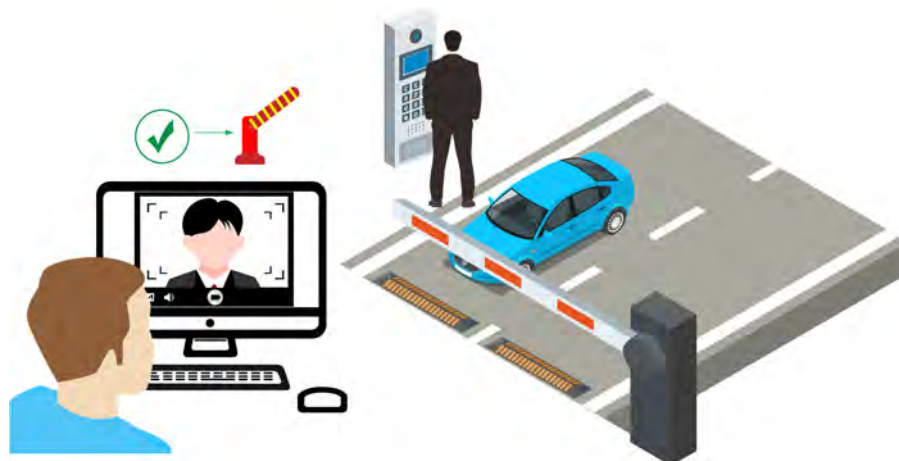
Figure 16-6 Opening Barrier by Video Intercom
