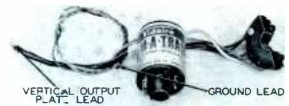
Fig. 7. ELIM-A-TRACE Used for Eliminating Vertical Retrace.
