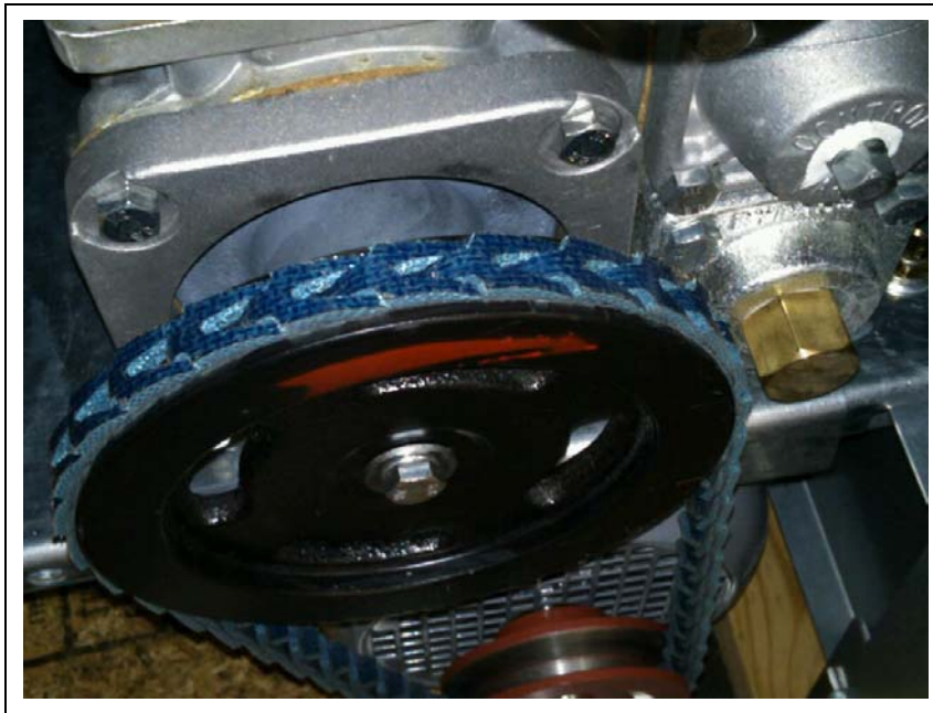
Figure C-5: Aligning the V-belt
