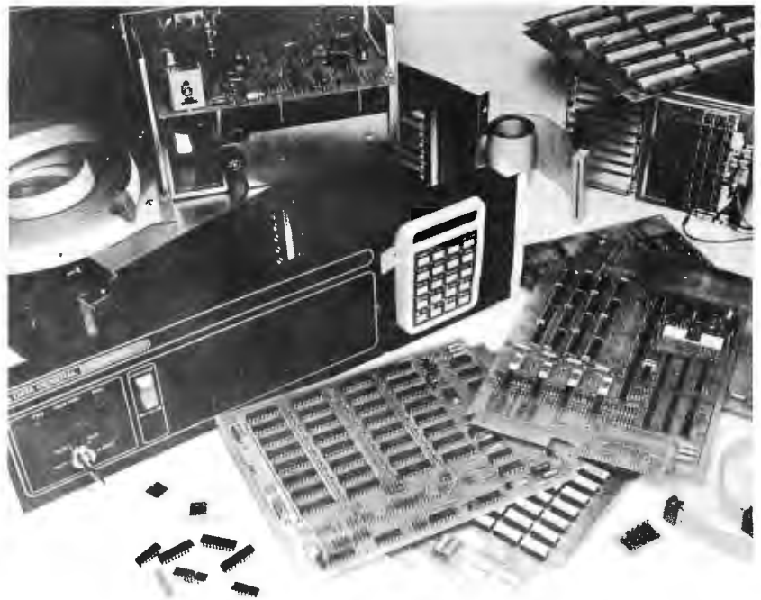
Photo 3: For the do it yourself systems house, Data General provides a complete line of modular components which can be integrated to form a microNOVA system. One of the most interesting characteristics of the microNOVAs integrated to the minicomputer level is a "Programmer's Helper" remote console packaged in a calculator style case at the end of a ribbon cable. The console is shown in its storage position in the front panel assembly at the center of this picture.
