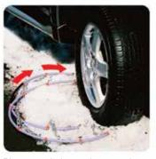
Place tyre chains on the ground facing the wheel. Slide chains around behind the "driving wheels," e.g: front wheel drive.
