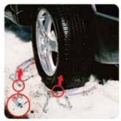
Locate the hook and chain, marked with multi-coloured washers (see inset photo).
