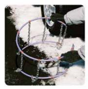
Hold tyre chains up and remove any twists so it hangs freely. Tip: Ensure the "blackband" is on the bottom hoop with the open end facing the wheel.
