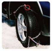
Lift hook and chain around the wheel and connect together at the top rear of the tyre.
