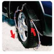
Keep rotating both plastic hoops around the wheel until the "blackband" sits at the top (front) of the tyre.
