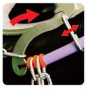
Ratchet the cam lever back and forth to increase the tension. Once tight, pull the cam lever back and secure it under the "side loop". Move vehicle forward 10m and readjust chains until they are very tight. Keep speed under 20kph.
