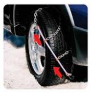
Start rotating both plastic hoops anti-clockwise around the wheel. Tip: Rotate both plastic hoops together.
