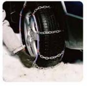
Shuffle the tyre chains around so they sit squarely on the tyre and then start tightening the chains around the wheel.
