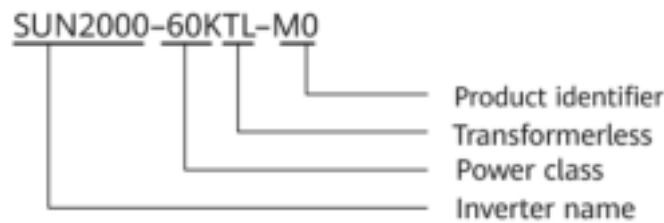
Figure 2-1 Designation explanation of the SUN2000-60KTL-M0
